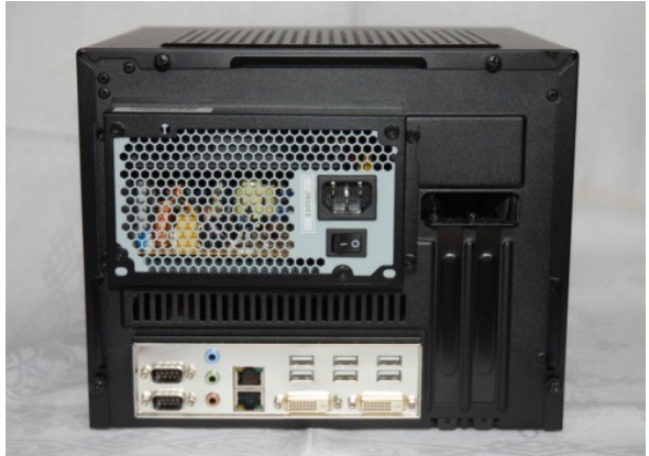
Rear view of Geoff's Titanium. The machine has two DVI ports and can drive two monitors. (Surprisingly for the editor, it does not have the more modern HDMI connections, which feed both video and audio to a monitor.) Six USB sockets, two gigabit network ports – and two serial ports – complete the array.
